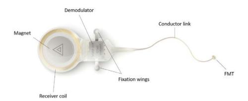
Figure 4. Vibrant Soundbridge - the VORP 503
