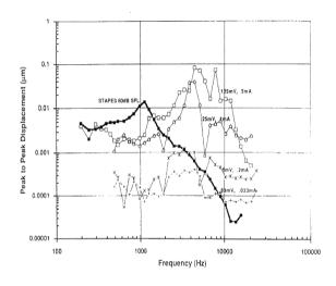
Figure 11. The frequency response of the first prototype transducer measured with an LDV in a temporal bone model (1993)
